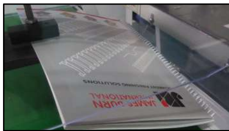
Automatic transport of the bound document onto a reception conveyor
