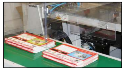
Head-to-tail reception to facilitate packing operations
