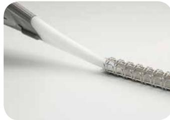
Position the nose of the RING WIRE OPENER into the wire seam.
