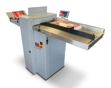
The maximum sheet size is 700mm x 385mm (900mm x 385mm with optional extension table) allowing a wider range of jobs to be tackled. Perforation is also standard on the DigiFold Pro with up to 5 perforation wheels being used across the sheet.
