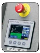
The new NCF6 control system with its Allen-Bradley Micro 850 PLC and Panelview C400 4.3 inch color touchscreen improves the operator interface, making it easy and fast to set up the machine or change sizes. Pre-programmed temperature and machine speed values are optimized for each coil diameter insuring consistent top quality coil while at the same time insuring MAXIMUM productivity.
