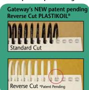
The reverse cut lead edge smoothly funnels its way through the punch hole in comparison to the standard cut lead edge. A great advantage especially when binding thicker books. An option on the PLASTIKOIL® New Concept Former. Retrofits also available for existing machines.
