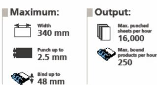
All performance outputs are based on 80 gam paper and may vary depending on the product type, the working environment and the operator. For best punching results we recommend a paper thickness of 1.5 - 2.0 mm.
