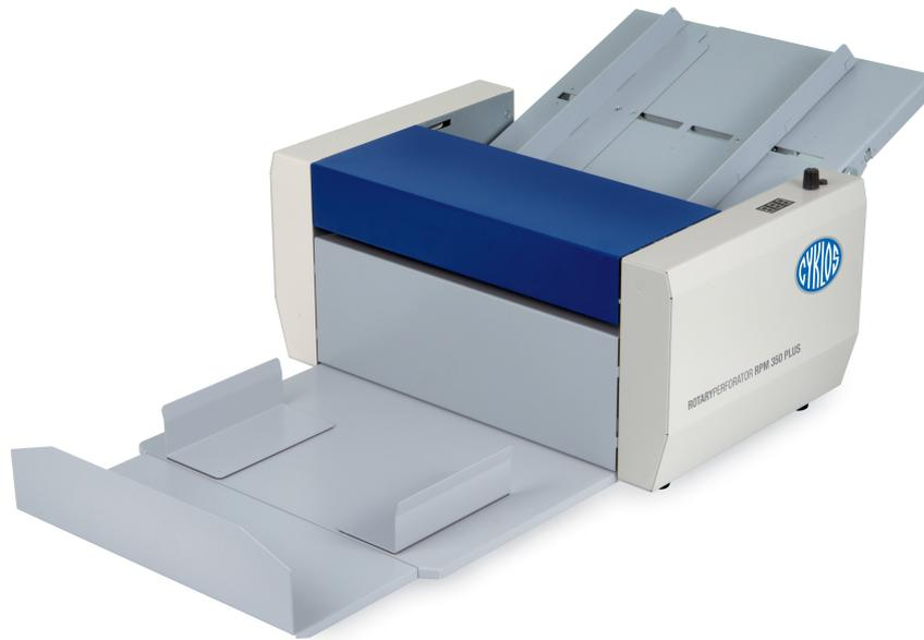
Dedicated auto perforating machine with auto friction feeding and a maximum working width of 350mm. Counter and speed control. Easy set up and operation. Sheets are quickly and easily perforated as they pass through sets of rotary perforating wheels.
