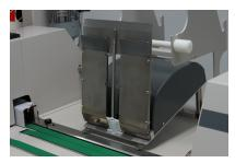
Optional automatic feeder for loose pre-formed hangers n°3 and n°7 with length from 76mm up to 250mm(up to 100 pieces)
